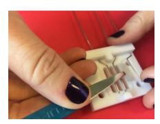
Push the wire and mesh into the groove using a small screwdriver or tweezers
