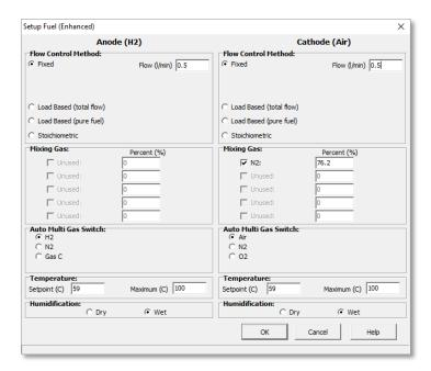
The FuelCell software will take care of the rest. It also works in load-based and stoichiometric flow rate controlled mode. FuelCell will vary the proportion of Air and pure  $N_2$  to get the final desired concentration of  $O_2$ .
