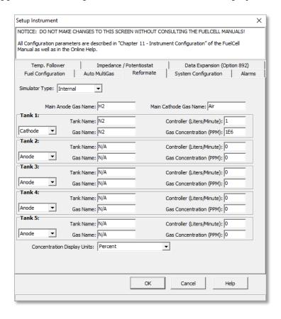
For a final gas mix of 5% O2, the Air needs to be diluted by a factor of 4.2x (= 21% / 5%). The fraction of pure N2 flow is then 76.2%:
