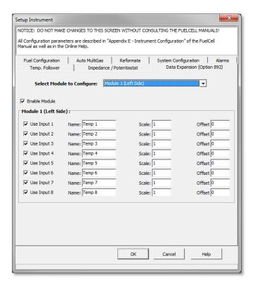
The **Data Expansion** tab is used to configure one or more Model 892 Data Expansion Units for use with an 890 or 850 system. See the 892 manual for additional information on the hardware.
