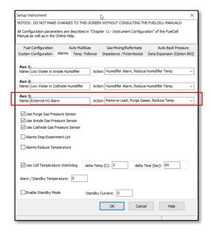
NOTE: The alarm-generating device should not produce any voltage on the 850's alarm input. It should only have a relay contact.
