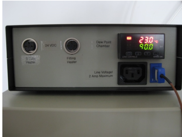
Figure 5. Front panel of the dew point chamber control box. The temperature controller controls the temperature of the dew point chamber. Note: The dew point chamber should be controlled to 10 °C above the maximum anticipated dew point ( i.e. , the dew point of the wet stream). The round connectors power the 24 V heaters used in the S-tube and the T-fitting copper clam shell.
