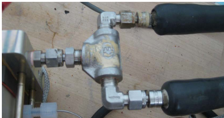
Figure 6. T-fitting connecting Anode (wet) and Cathode (dry) gas streams.
