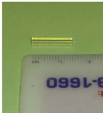
Figure 8. Preparation of 3 mm OD alignment pin tubing for use with a cell that incorporates flow frames.
