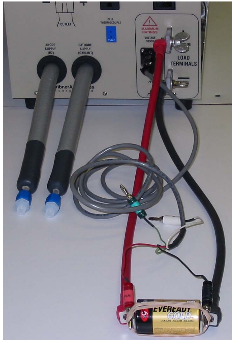
Figure 1 – Battery Connection to Test Station
